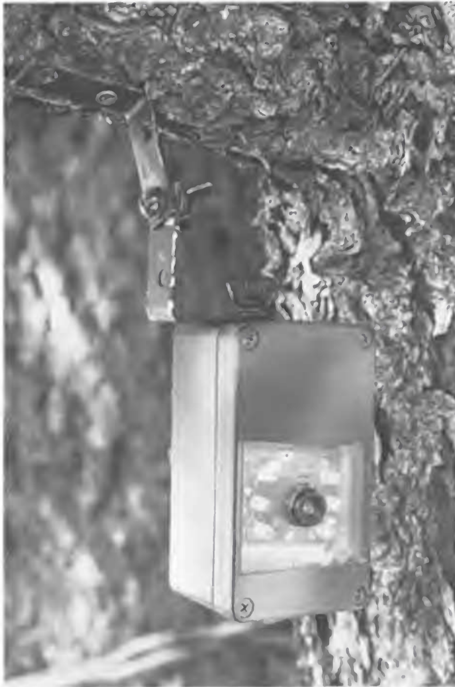
Figure 3. Branch-mounted video camera showing jointed attachment bracket, adjustable in two planes. Power and video cables are attached through connectors on the rear of the unit (not visible in this view) and anchored to the supporting branch or tree trunk.
